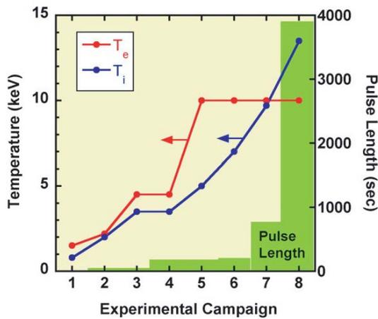
**Fig. 3.** (Color online) Progress of achieved electron, ion temperatures, and pulse length of discharge.
