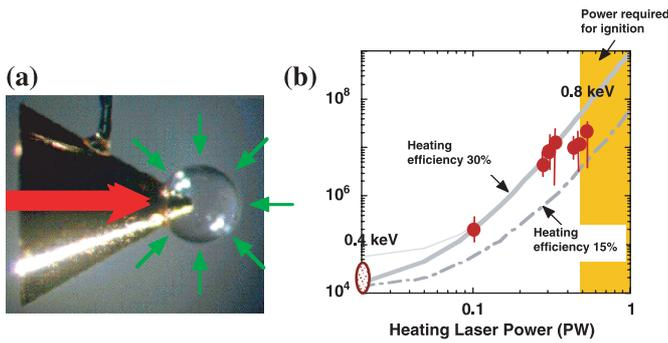
**Fig. 6.** (Color online) (a) A fuel shell attached with a gold cone for laser entry; (b) DD neutron yield as a function of the heating laser power [11].
